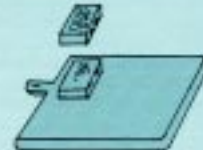
Fig. B insert the solar cells in the correct circuit format in the plastic tray
