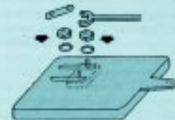
Fig. C position the copper links in the correct circuit format and tighten screws
